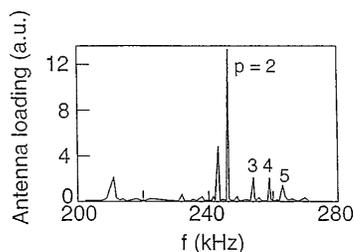
FIG. 5. Antenna-driven spectra computed by the PENN code for shot 33157 at  $t = 19$  s.
