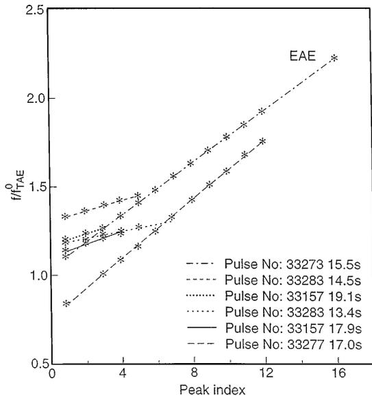
FIG. 3. Example of frequency distribution of the multiple AE driven by an external antenna for a number of additionally heated JET discharges. The peak index enumerates the AE from the lowest frequency peak observed in the TAE range.
