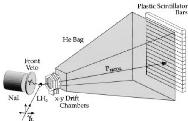
FIG. 1. Schematic arrangement used to identify  $\gamma$ -proton coincidences, with photons measured in a NaI(Tl) crystal and protons in an array of scintillator bars.
