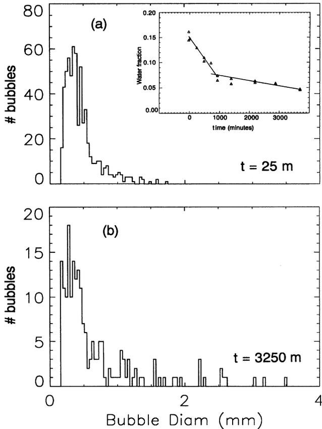
FIG. 2. Bubble size distribution at successive times of same cross section as Fig. 1 (a) at  $t = 25$  min, (b) at  $t = 3250$  min. Note the extended tail of large bubbles in (b). Inset: liquid fraction in foam slice vs time. Linear fits to drainage rates are superposed.
