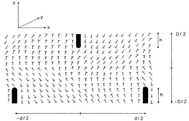
FIG. 5. The director modulation in the free suspended film of the thickness  $D$  in ferroelectric Sm-C phase. The in-plane modulation between the walls of height  $h$  has periodicity  $d$ . The director azimuthal angle  $\Omega_z$  varies continuously by  $\pi$  between the walls and jumps by  $\pi$  at the walls. The surfaces are connected by the director twist along the smectic layer normal.
