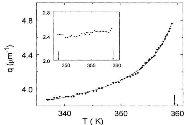
FIG. 3. Temperature dependence of the stripe periodicity wave vector  $q$  in Cl 8/5 measured in  $\sim 10 \mu\text{m}$  thick film. The line is a power law fit with the critical exponent 0.5. In the inset the temperature dependence of  $q$  in MHPOBC is shown. The arrows indicate transition temperatures between the stripe and homeotropic textures.
