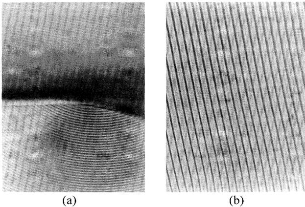
FIG. 1. (a) The texture at the transition between the homeotropic and stripe phase in Cl 8/5 at 82 °C, the stripe periodicity  $d = 1.3 \mu\text{m}$ ; (b) the stripe texture in MHPOBC at 80 °C,  $d = 2.5 \mu\text{m}$ . The lower and upper lines mutually shifted by  $d/2$  are visible in a different contrast.
