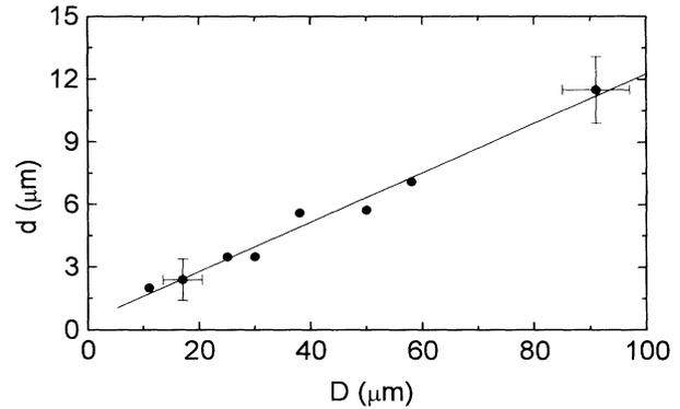
FIG. 2. Thickness dependence of the stripe periodicity  $d$  in Cl 8/5 doped with 10% of a nonchiral Sm-C. The nonchiral dopand was used to increase  $d$  for easier microscopic measurements. The line is the fit to the theoretical solution  $d(D)$ .
