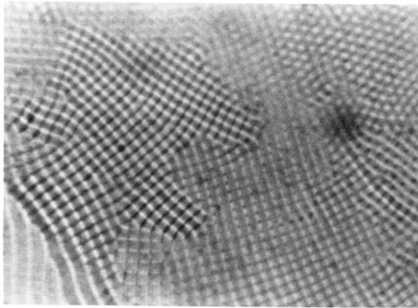
FIG. 7. The 2D patterns observed in the temperature gradient. The consecutive hexagonal→square→stripe texture transitions are observed under the temperature decrease.
