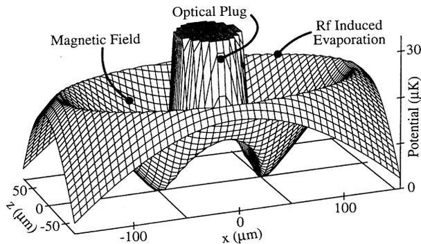
FIG. 1. Adiabatic potential due to the magnetic quadrupole field, the optical plug, and the rf. This cut of the three-dimensional potential is orthogonal to the propagation direction ( $y$ ) of the blue-detuned laser. The symmetry axis of the quadrupole field is the  $z$  axis.
