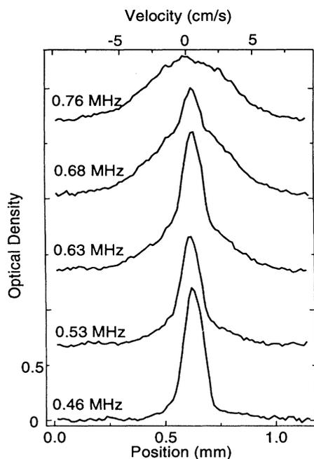
FIG. 3. Optical density as a function of position along the  $z$  axis for progressively lower values of the final rf frequency. These are vertical cuts through time-of-flight images like those in Fig. 2. For  $\nu_{\text{rf}} < 0.7$  MHz, they show the bimodal velocity distributions characteristic of the coexistence of a condensed and uncondensed fraction. The top four plots have been offset vertically for clarity.
