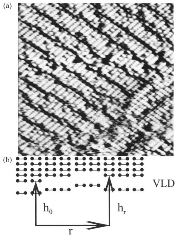
FIG. 1. (a) High-resolution STM image of a Ni (a few percent of a monolayer) contaminated Si(001) surface. The scan size is  $25 \text{ nm} \times 25 \text{ nm}$ , the sample bias  $-2 \text{ V}$  and the tunneling current  $0.5 \text{ nA}$ . (b) Schematic representation of a VLD.  $h$  and  $r$  are measured in units of  $a$  and  $2a$ , respectively ( $a = 3.84 \text{ \AA}$ ).
