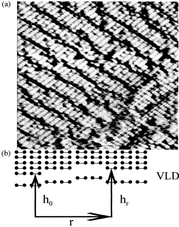
FIG. 1. (a) High-resolution STM image of a Ni (a few percent of a monolayer) contaminated Si(001) surface. The scan size is  $25 \text{ nm} \times 25 \text{ nm}$ , the sample bias  $-2 \text{ V}$  and the tunneling current  $0.5 \text{ nA}$ . (b) Schematic representation of a VLD.  $h$  and  $r$  are measured in units of  $a$  and  $2a$ , respectively ( $a = 3.84 \text{ \AA}$ ).
