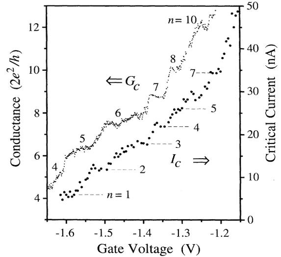
FIG. 2. The critical current  $I_c$  and the constriction conductance  $G_c$  as a function of the gate voltage  $V_g$ . All measured critical-current steps from the first to the seventh step are shown as well as the corresponding conductance steps from the fourth to the tenth.
