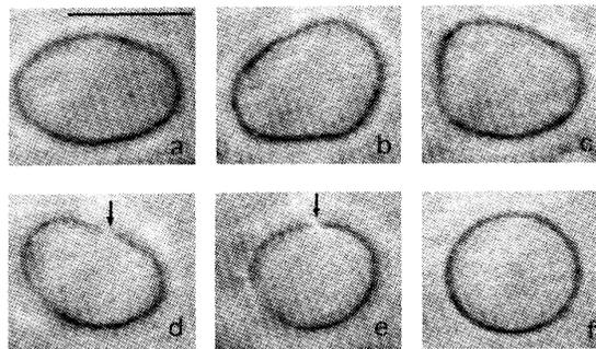
FIG. 1. *Optically induced pressure in a vesicle.* The vesicle was seen to fluctuate strongly at first (a)–(c), then as the optical tweezers were applied (d),(e) the fluctuations gradually decreased until the vesicle became tense (f). It took about 100 sec for the pressurization to be completed. The pressurized vesicle was observed to be unchanged over several hours. The bar represents 10  $\mu\text{m}$ .
