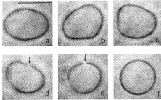
FIG. 1. *Optically induced pressure in a vesicle.* The vesicle was seen to fluctuate strongly at first (a)–(c), then as the optical tweezers were applied (d),(e) the fluctuations gradually decreased until the vesicle became tense (f). It took about 100 sec for the pressurization to be completed. The pressurized vesicle was observed to be unchanged over several hours. The bar represents 10  $\mu\text{m}$ .
