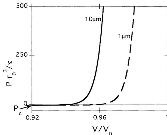
FIG. 3. *Laser induced tension and pressure in vesicles.* The equation of state of pressurized vesicles. Pressure-volume isotherms are given for two relevant vesicle radii.
