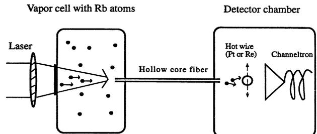
FIG. 1. Experimental apparatus. Laser light is coupled into the grazing incidence modes of a hollow-core fiber. Atoms with small transverse velocities are extracted from a vapor cell in the first chamber and guided through the hollow fiber to a detection chamber.
