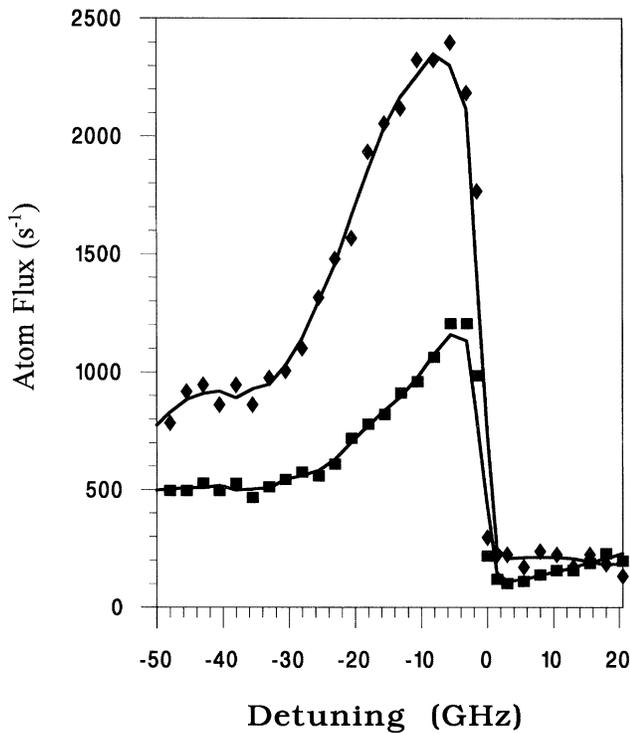
FIG. 2. Guided atom signal versus laser detuning from resonance. For the upper curve,  $I_0 = 3.6 \times 10^3 \text{ W/cm}^2$  in the guiding modes, and for the lower curve,  $I_0 = 1.3 \times 10^3 \text{ W/cm}^2$ . The data show a sharp increase in the guided atom signal when the laser is tuned slightly to the red of the  $D2$  resonance line of Rb. The solid line is included to show the trend of the data.
