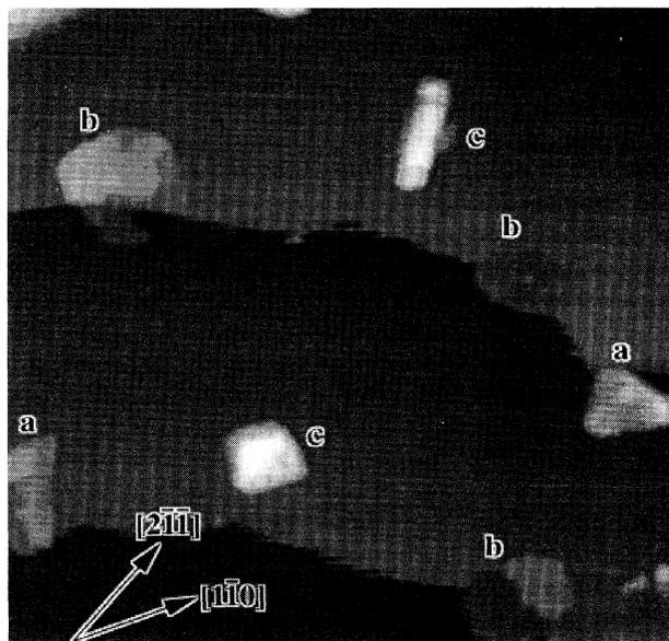
FIG. 1. STM image of Pb(111) after deposition of 0.94 ML Cu. Three different types of Cu islands are visible ( $100 \times 100$  nm<sup>2</sup>).
