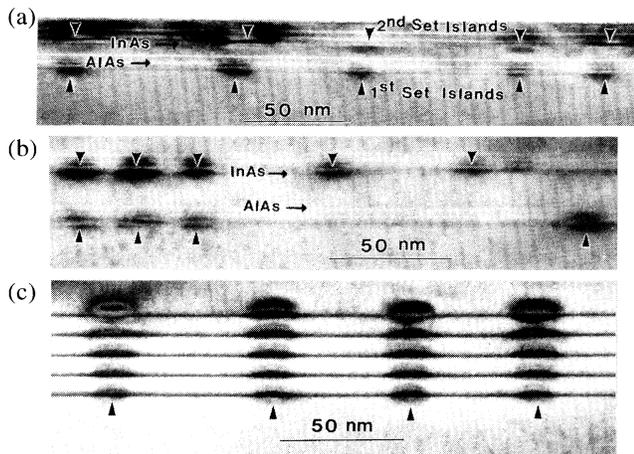
FIG. 1. Typical  $g = (400)$  bright field TEM pictures taken along  $[011]$  azimuth for the samples with two sets of islands separated by (a) 46 and (b) 92 ML spacer layers, respectively. Arrows point to the island positions indicated by the strain contrast. (c) A typical  $g = (200)$  dark field TEM picture for a sample with five sets of islands separated by 36 ML spacer layers. Note the vertical collinearity of the islands in five sets.
