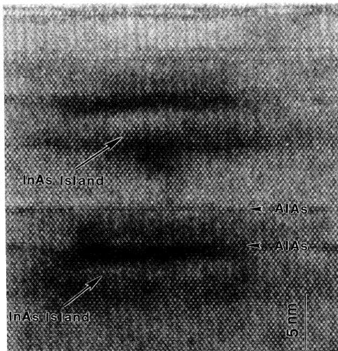
FIG. 2. High resolution lattice image taken with  $[011]$  azimuth for the sample with 46 ML spacer shows the vertical correlation and coherent nature of the islands. The first and second AIAs marker layers and the GaAs profile for the deposition of the second InAs layer are seen to be flat.
