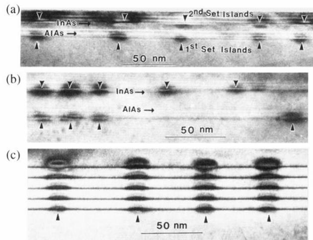
FIG. 1. Typical  $g = (400)$  bright field TEM pictures taken along  $[011]$  azimuth for the samples with two sets of islands separated by (a) 46 and (b) 92 ML spacer layers, respectively. Arrows point to the island positions indicated by the strain contrast. (c) A typical  $g = (200)$  dark field TEM picture for a sample with five sets of islands separated by 36 ML spacer layers. Note the vertical collinearity of the islands in five sets.
