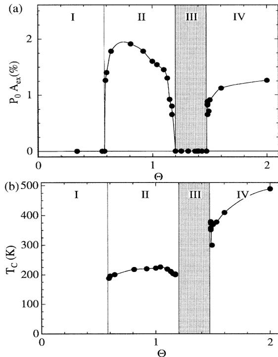
FIG. 3. (a) Maximum values of  $P_0 A_{\text{ex}}$  observed for temperatures  $T > 115$  K versus Fe coverage  $\theta$ . (b) Curie temperatures  $T_c$  versus  $\theta$ . Regimes I–IV are as discussed in the main text. The gap of long range order in regime III is obvious.
