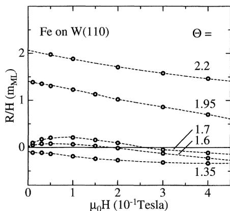
FIG. 5. Torsion oscillation magnetometry of Fe(110) films on W(110) at 300 K.  $R/H$  (magnetic torque constant  $R$  per magnetic field  $H$ ), in units of  $m_{ML}$  (the saturation moment of a pseudomorphic monolayer with  $2.17\mu_B$  per atom), versus  $H$  which is applied along [110].
