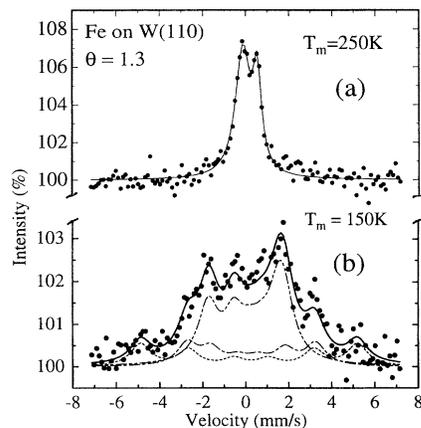
FIG. 4. CEMS spectra of a pure  $^{57}\text{Fe}$  film on W(110),  $\theta = 1.3$ , prepared at 300 K, and measured in zero field (a) at 250 K and (b) at 150 K.
