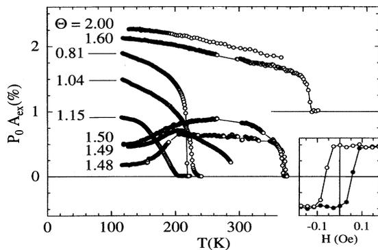
FIG. 2. Exchange asymmetry  $P_0 A_{\text{ex}}$  versus temperature  $T$  for Fe(110) films on W(110), with coverage  $\theta$  as a parameter. The inset shows the magnetization loop for a film  $\theta = 1.48$ , 10 K below  $T_c$ .
