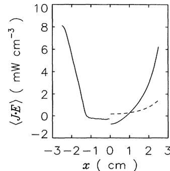
FIG. 5. Comparison of the time-averaged heating  $\langle JE \rangle$  obtained from the periodic simulation (left half of the figure) with the result of the theory discussed in the text (right half of the figure). The dotted line in the right half of the figure is the Ohmic component of the heating calculated from the theory.
