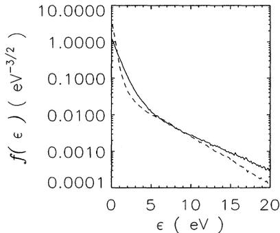
FIG. 2. A comparison of the electron energy distribution functions from the bounded simulation and the analogous periodic model system, for the same conditions as in Fig. 1. These data are time averaged at  $x = 0$ . The solid and dashed lines are from the bounded and periodic models, respectively.
