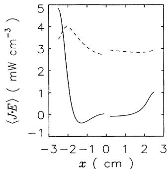
FIG. 6. Comparison of the numerical solutions of essentially Eqs. (1) and (2), with and without the flux-limited thermal conductivity. The left half of the figure shows the flux-limited case, the right half the conventional solution. Solid lines denote  $\langle JE \rangle$  and dashed lines are  $T_e^{(0)}(x)$  expressed in arbitrary units. In both cases  $T_e^{(0)}(x=0) \approx 3$  eV. Except as noted in the text, the conditions are the same as in Figs. 3 and 5.
