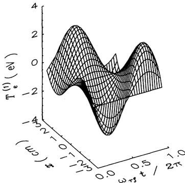
FIG. 3. A sample solution of Eq. (4) of the text, showing the thermal wave. The parameters (using symbols defined in the text) are  $n_0 = 6 \times 10^8 \text{ cm}^{-3}$ ,  $J_0 = 1 \text{ mA cm}^{-2}$ ,  $T_0 = 3 \text{ eV}$ ,  $x_0 = 0.8 \text{ cm}$ ,  $x_1 = 0.9 \text{ cm}$ ,  $\omega_{rf} = 2\pi \times 13.56 \text{ MHz}$ ,  $\bar{\nu}_e = 60 \text{ MHz}$ , and  $L = 2.5 \text{ cm}$ . The phase is referenced to  $J(t) = J_0 \sin \omega_{rf} t$ .
