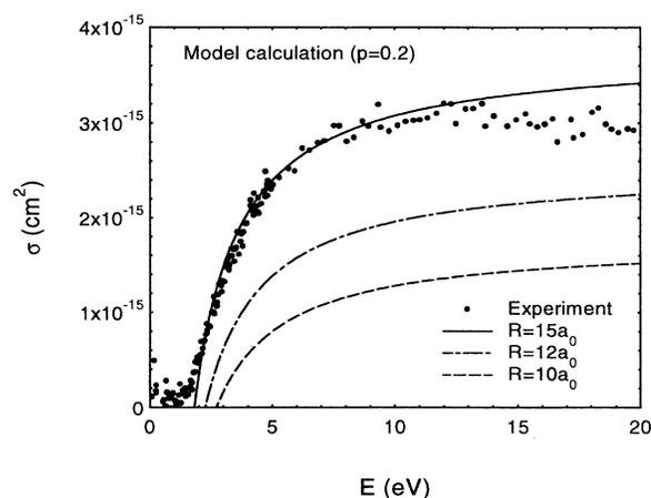
FIG. 3. Electron-impact detachment cross section of  $D^-$  as a function of energy. The model calculation is compared with the experimental data for three different values of reaction radius  $R$ .
