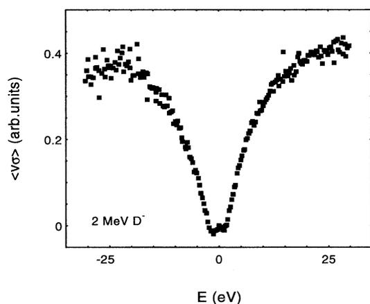
FIG. 2. Rate coefficient  $\langle v\sigma \rangle$  as a function of the relative energy ( $E < 0$  for  $v_e < v_i$  and  $E > 0$  for  $v_e > v_i$ , where  $v_e$  and  $v_i$  are the electron and ion velocity, respectively). The ion-beam energy was 2 MeV; the electron density at  $E = 0$  was  $7 \times 10^5 \text{ cm}^{-3}$ .
