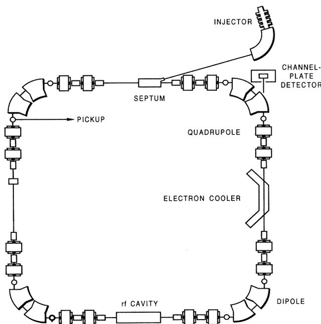
FIG. 1. Schematic drawing of the storage ring ASTRID. The electron cooler is used as the electron target (interaction length of 85 cm).
