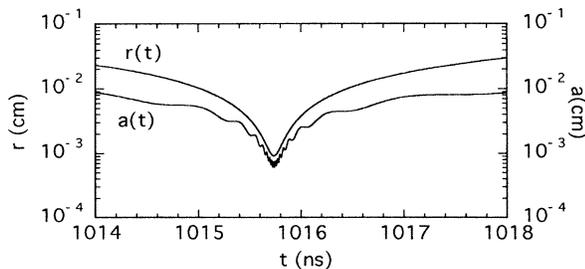
FIG. 3. Plots of the outer pinch radius and the inner fiber radius as a function of time during the last phase of compression.
