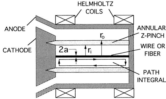
FIG. 1. Schematic illustration of the staged Z-pinch configuration.
