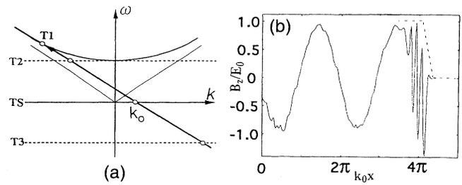
FIG. 2. Dispersion diagram (a) for electromagnetic, electrostatic, and free streaming plasma modes intersected by line of constant phase; and 2D particle-in-cell simulation (b) of  $B_z/E_0$  (solid) and plasma density  $n/n_{\max}$  (dashed) vs  $k_0 x$  for a continuous front located at position  $k_0 x = 13.8$  and length  $0.4/k_0$ .
