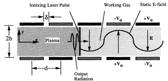
FIG. 1. Schematic of dc to ac light converter.
