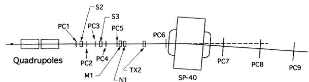
FIG. 2. Schematic layout of spectrometer Anomalon. SP40, analyzing magnet; PC1-7, three-dimensional ( $X, U, V$ ) MWPCs; and PC8,9, two-dimensional ( $X, Y$ ) MWPCs; S2, S3, N1, M1, TX2, trigger and TOF scintillation counters.
