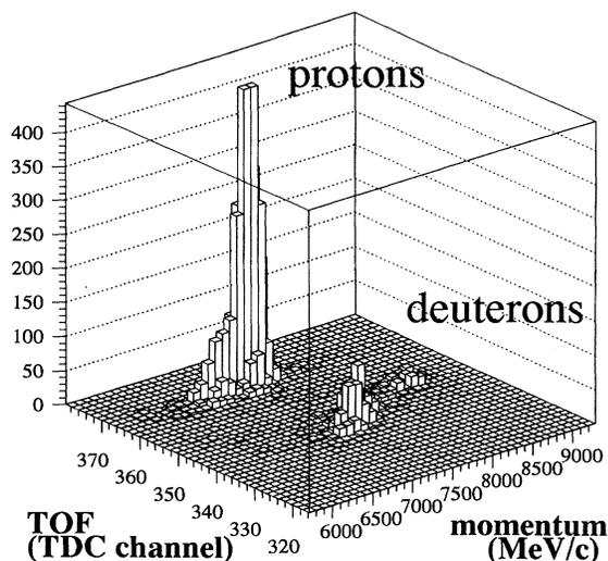
FIG. 3. The two-dimensional plot of TOF versus momentum for the detected events at the deuteron beam momentum 8.7 GeV/c and the beam line momentum 7.5 GeV/c. The TOF time scale (one digit of the TDC) was 220 ps/channel.
