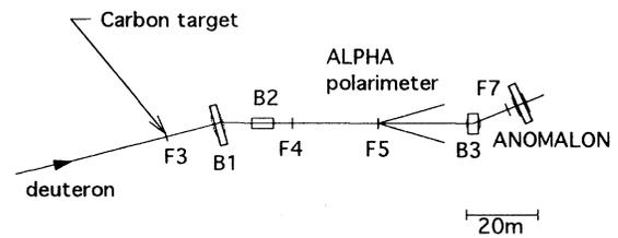
FIG. 1. Schematic layout of the beam line.  $B$  denotes the bending magnets.  $F3, F4, F5$ , and  $F7$  are the focusing points.
