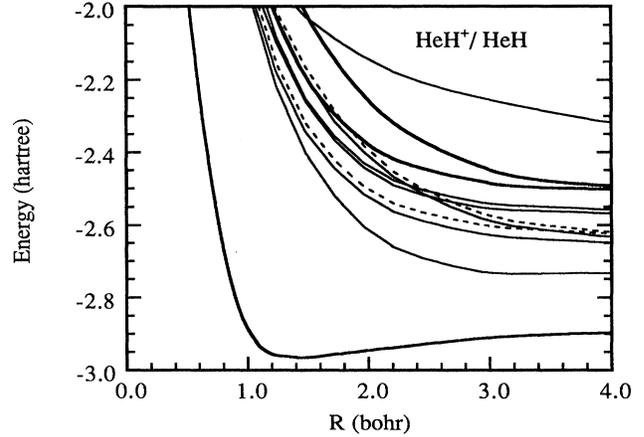
FIG. 2. Potential energy curves of  $\text{HeH}^+$  and  $\text{HeH}$  relevant to the present study. The  $X^1\Sigma^+$ ,  $a^3\Sigma^+$ , and  $A^1\Sigma^+$  ion curves are the heavy solid curves. The thin solid curves are the  $^2\Sigma$  neutral resonance states and the dashed curves are the  $^2\Pi$  states.
