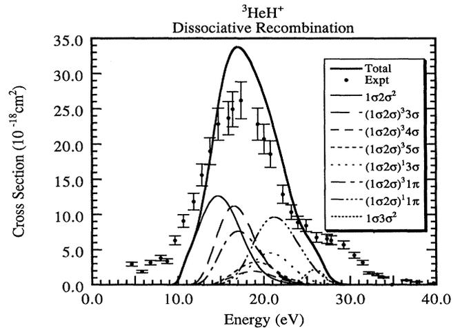
FIG. 3. Total (heavy solid curve) and partial DR cross sections for ground-state  $^3\text{HeH}^+$  as a function of incident electron energy. The experimental points are those of Sundström *et al.* (Ref. [10]).
