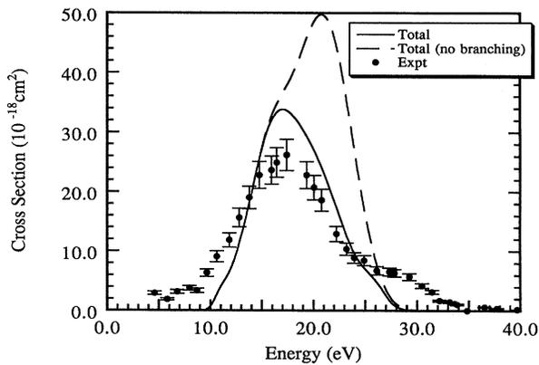
FIG. 4. Sensitivity of computed DR cross section to the neglect of partial widths to excited ion channels. The dashed curve is obtained by using the total widths to compute the entry amplitudes.
