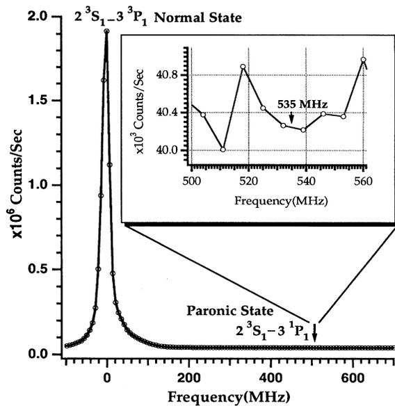
FIG. 3. Fluorescence spectrum scanned over the region of interest. The inset shows a greatly magnified view of the region of the spectrum which would produce a line if PEP were violated.
