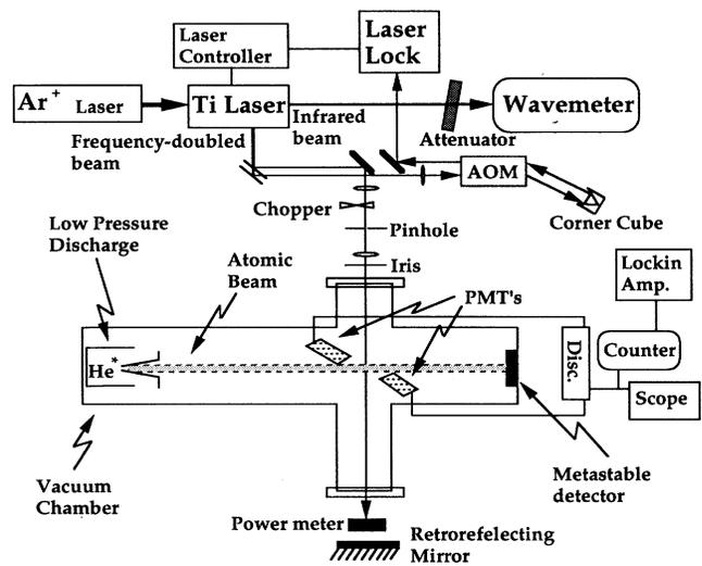
FIG. 2. Schematic diagram of the apparatus.
