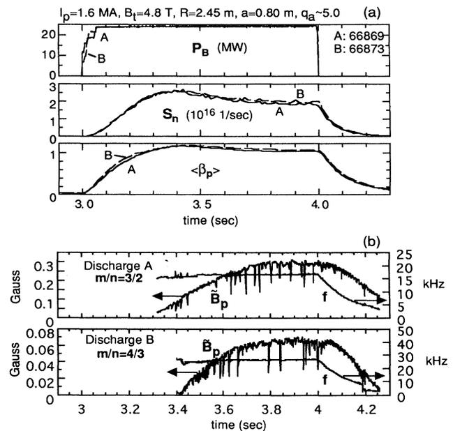
FIG. 1. (a) Two typical supershot discharges with different MHD modes. Here,  $P_B$  is the neutral beam power,  $S_n$  is the total DD neutron rate, and  $\langle \beta_p \rangle$  is the volume-averaged poloidal beta. (b) Discharge A has a dominant  $m/n = 3/2$  mode. Discharge B has a  $4/3$  mode. The mode amplitude ( $\tilde{B}_p$ ) and frequency ( $f$ ) are measured by a Mirnov coil.
