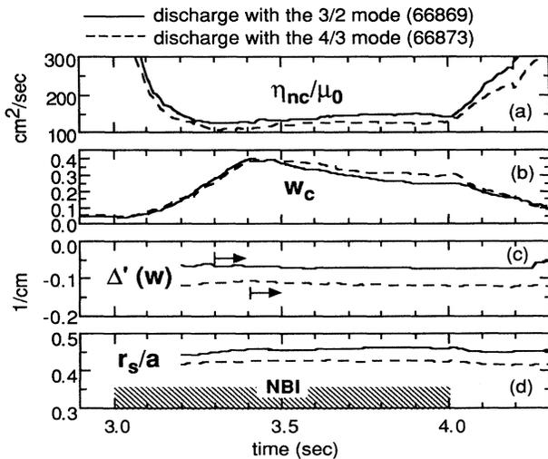
FIG. 3. The time evolution of the parameters used in Eq. (1). (a) Magnetic field diffusivity  $\eta_{nc}/\mu_0$ . (b) Neoclassical driving term  $w_c$ , Eq. (2). (c) Numerically calculated  $\Delta'(w)$  [Eq. (7)]. (d) Mode location. The arrows indicate the time when the MHD mode begins.
