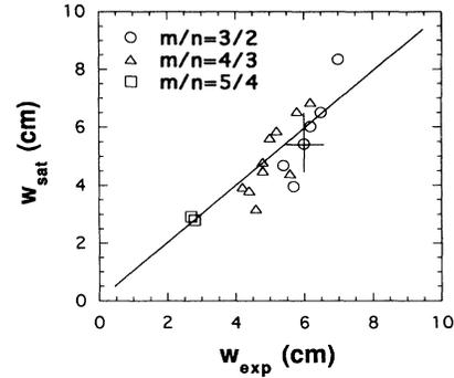
FIG. 4. Theory-experiment comparison of saturated magnetic island width. The  $w_{exp}$  is from Eq. (5). The  $w_{sat}$  is from Eq. (4). A constant  $k_2 = 1.7$  has been used for all discharges.
