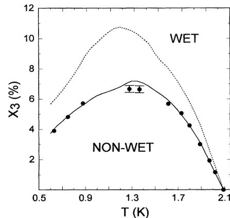
FIG. 2. The  $X_3$  vs  $T_w$  wetting phase diagram for  $^3\text{He}$ - $^4\text{He}$  mixtures on Cs. The dashed curve is calculated from Eq. (1) assuming no bound state at the He-Cs interface. The solid curve is a best fit and includes a  $^3\text{He}$  state at the He-Cs interface with a binding energy of 1.95 K. In the region below the curve the cesium surface is nonwet. Above the curve it is wet.
