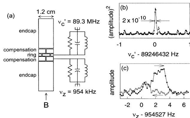
FIG. 2. Open access Penning trap electrodes and detection circuits in (a), with the cyclotron (b), and axial (c) signals from one trapped  $\bar{p}$ .
