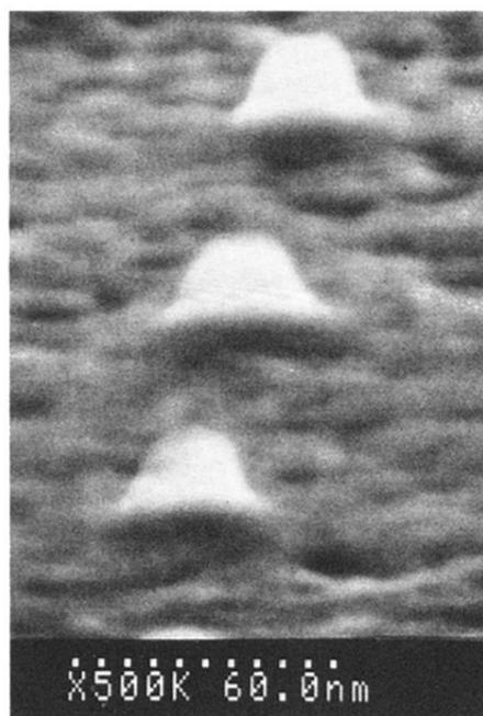
FIG. 1. Scanning electron micrograph of 30 nm  $\text{In}_{0.13}\text{Ga}_{0.87}\text{As}/\text{GaAs}$  quantum dots.
