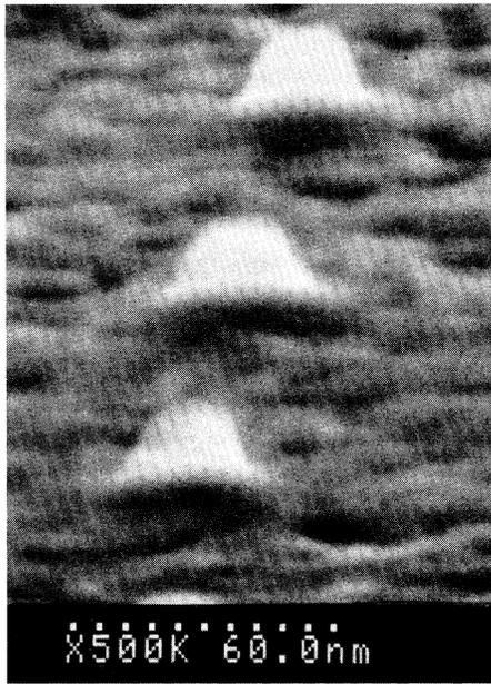
FIG. 1. Scanning electron micrograph of 30 nm  $\text{In}_{0.13}\text{Ga}_{0.87}\text{As}/\text{GaAs}$  quantum dots.
