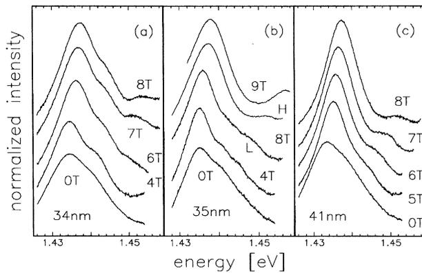
FIG. 3. High excitation photoluminescence spectra at varying magnetic fields for dots of 34 nm diameter (a), for dots of 35 nm diameter (b), and for dots of 41 nm diameter (c). The laser excitation power was  $7.5 \text{ kW cm}^{-2}$  except for the two topmost spectra of the 35 nm dots at  $B = 8 \text{ T}$  (*H*) and at  $B = 9 \text{ T}$ , where an excitation power of  $15 \text{ kW cm}^{-2}$  was used.
