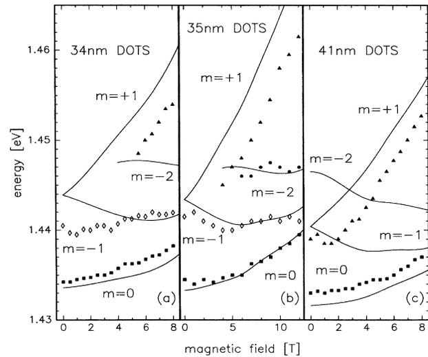
FIG. 4. Magnetophotoluminescence results for the ground state and higher lying transitions as functions of the magnetic field for modulated barrier dots with diameters of 34 nm (a), 35 nm (b), and 41 nm (c). The solid lines give the results of the calculations.
