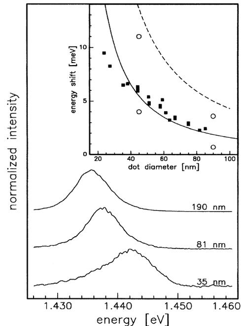
FIG. 2. Photoluminescence spectra of quantum dots with diameters of 35, 81, and 190 nm. The inset shows the measured shifts of the lowest transitions in photoluminescence as functions of dot size. The solid and dashed curves give the results of calculations described in the text. The open circles denote data obtained by photoluminescence excitation spectroscopy.
