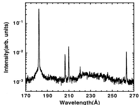
FIG. 1. MCPIGS on-axis spectrum obtained in the Nova experiments from 3 cm long targets of Se illuminated by a series of three 100 ps pulses 400 ps apart with peak intensity of  $110 \text{ TW}/\text{cm}^2$ . The Ne-like  $J = 0 \rightarrow 1$  laser line at 182 Å dominates the spectrum. The  $J = 2 \rightarrow 1$  lines at 206 and 209 Å as well as the other laser lines at 220 and 262 Å are quite visible.
