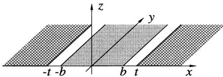
FIG. 1. The model of the split-gate device. The two shaded areas represent the gate in the shape of two semi-infinite planes. Beneath the gate the two-dimensional electron gas located in  $z = 0$  plane is depleted. The density of the electron gas does not vanish only in a narrow strip (grey area) between the two halves of the gate.
