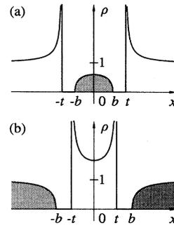
FIG. 2. The optimal eigenvalue density fluctuation  $\rho(x)$  for (a)  $n < s$ , (b)  $n > s$ . The grey and blank regions show the locations of the 2DEG charge and the gate charge, respectively, in the equivalent gated devices. given by the expression
