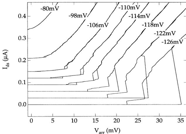
FIG. 2. Typical  $I$ - $V$  curves for several gate voltages (device 2) measured at base temperature ( $T \sim 20$  mK). The curves are offset in proportion to gate voltage ( $V_g$ ) for clarity.  $V_{arr}$  is the voltage measured directly across the array in a four-lead configuration.
