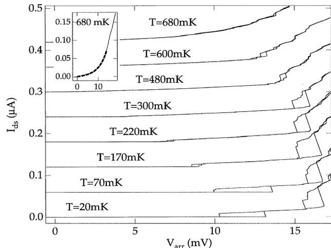
FIG. 3.  $I$ - $V$  curves (offset for clarity) for device 2 at  $V_g = -115$  mV at various temperatures. Inset shows finite conductance around zero bias for higher temperature data ( $T = 680$  mK) (solid curve) on enlarged vertical scale, along with a two-parameter fit by the activated form  $I_{ds} = K_1 \sinh(K_2 V_{arr})$  (dashed curve). Fit gives  $K_1 = 3.4$  nA and  $K_2 = 0.27$  mV $^{-1}$ .
