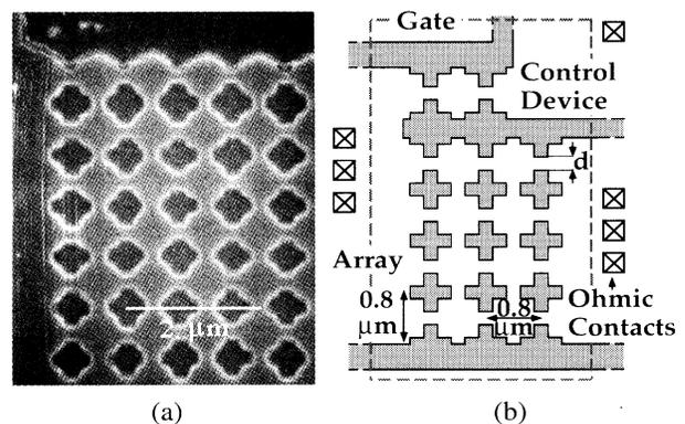
FIG. 1. (a) Electron micrograph of part of the  $200 \times 200$  array. Electron gas is removed beneath darker regions; channels between dots can be depleted with a gate voltage in the range  $-40$  to  $-150$  mV depending on the device. (b) Schematic shows the layout of the array, control device, and Ohmic contacts. The lithographic distance “ $d$ ” is 300, 250, and 200 nm for device 1, 2, and 3, respectively.
