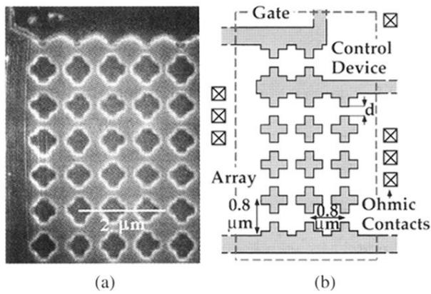
FIG. 1. (a) Electron micrograph of part of the  $200 \times 200$  array. Electron gas is removed beneath darker regions; channels between dots can be depleted with a gate voltage in the range  $-40$  to  $-150$  mV depending on the device. (b) Schematic shows the layout of the array, control device, and Ohmic contacts. The lithographic distance " $d$ " is 300, 250, and 200 nm for device 1, 2, and 3, respectively.
