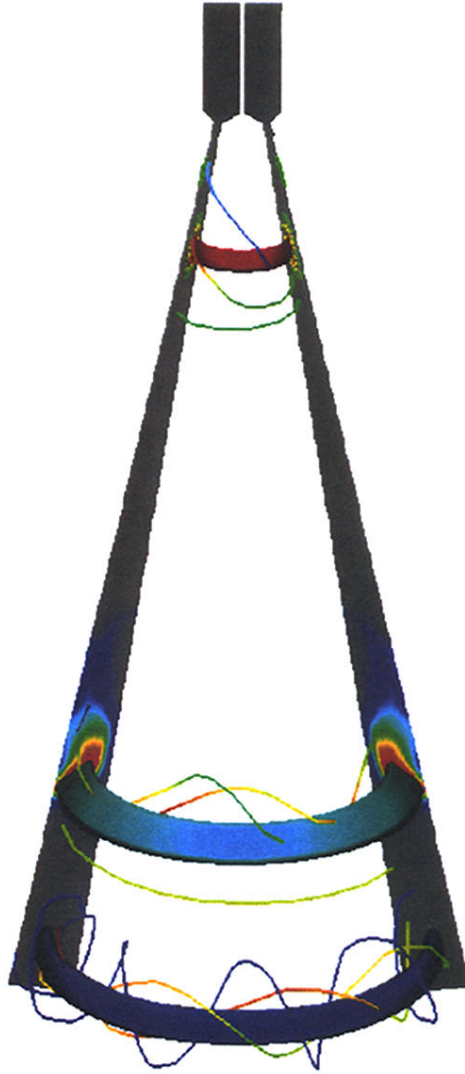
FIG. 4. Superposition of snapshots of the mass density and magnetic field lines of a CT at t = 0, 3.0 and 6.0 \mu s in a long converging geometry that is designed to achieve a final speed of 10^9 m/s in 6.5 \mu s . Three magnetic field lines from the initial toroid are shown to twist around a mass density isosurface (blue). The later-time data each have an almost purely azimuthal field line located upstream of the CT that represents the piston field. The mass density increases with time (red is higher density than blue).
