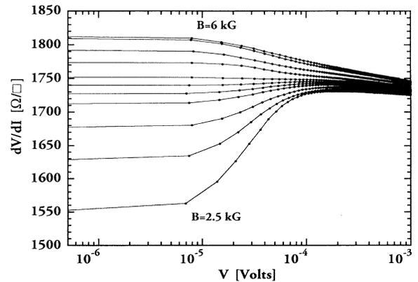
FIG. 2. Dynamical sheet resistance measured for sample 2 as a function of the bias voltage at 70 mK for  $B = 2.5, 3.0, 3.4, 3.8, 4.0, 4.2, 4.4, 4.8, 5.4, 5.9, 6$  kG.
