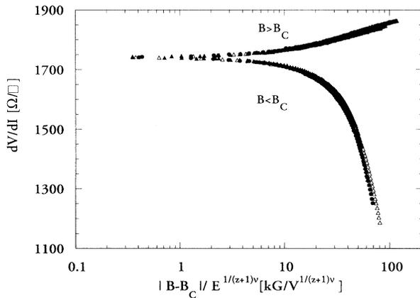
FIG. 4. Scaling of the  $\delta V/\delta I$  for sample 2 measured at  $T = 70$  mK [ $B_c = 4.19$  kG,  $\nu(z+1) = 2.73$ ].
