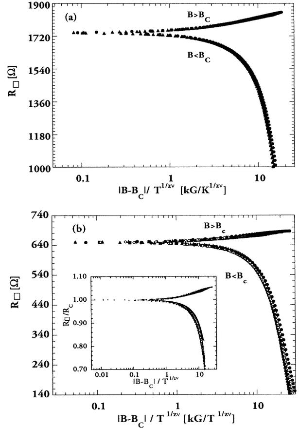
FIG. 3. Top: Scaling of  $R_{\square}(B, T, E=0)$  for sample 2 measured at  $T = 80, 90, 100, 110$  mK ( $B_c = 4.19$  kG,  $\nu z = 1.36$ ). Bottom: Scaling for sample 5 of the data measured at  $T = 100, 200, 300, 400$  mK ( $B_c = 25.6$  kG,  $\nu z = 1.36$ ). Bottom inset:  $R_{\square}/R_c$  versus the scaling variable for samples 2 and 5 together.
