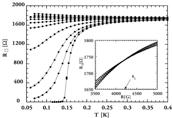
FIG. 1. Zero bias resistance of sample 2 plotted versus temperature at  $B = 0, 0.5, 1.0, 2.0, 3.0, 4.0, 4.4, 4.5, 5.5, 6$  kG. In the inset,  $R_{\square}(B, T, E = 0)$  for the same sample measured versus field, at  $T = 80, 90, 100, 110$  mK.
