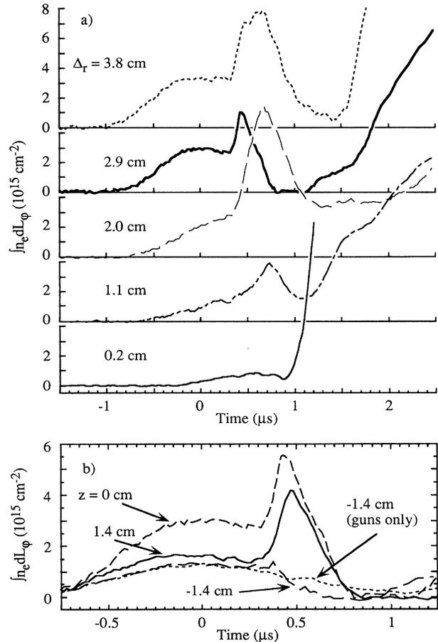
FIG. 3. (a) Line plasma density measured at different  $\Delta_r = r - r_c$  along the gun axis. (b) Analogous measurements for different distances from the gun axis  $z$  at 2.9 cm from the cathode. The guns-only line density time behavior at  $z = -1.4 \text{ cm}$  is also shown. Zero time corresponds to the upstream current beginning.
