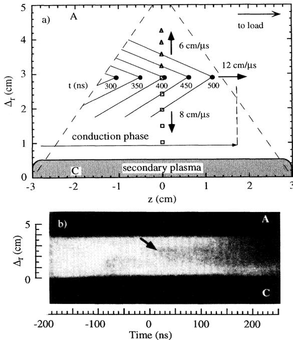
FIG. 4. (a) Reconstruction of the density maximum propagation through the plasma. Dashed lines indicate the initial plasma boundary. Moments of the peak maximum arrival are referred to the start of the upstream current. (b) Visible streak picture of the plasma (gun axis). The arrow points to the wedge front. Zero time corresponds to the 10% amplitude of the load current.
