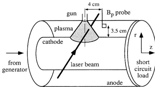
FIG. 1. A sketch of the experimental arrangement.
