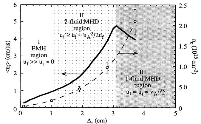
FIG. 5. Radial dependence of the function  $\langle u_i(r) \rangle$  (see text) behind the KMC-type magnetic field shock (I, II) and due to the snow-plow plasma pushing (III). Electron density is calculated for the moment of the upstream current beginning as  $n_e = \langle n_e L_p \rangle / L_p$ , where  $L_p(r)$  was obtained by scanning the plasma in axial direction [9].
