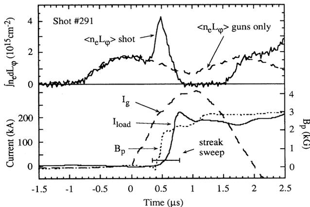
FIG. 2. Measured line integrated density for the position 2.9 cm from the cathode and 1.4 cm from the gun axis towards the load.  $L_\phi$  denotes one plasma length (2.8 cm). Also shown are upstream ( $I_g$ ) and downstream ( $I_{load}$ ) currents,  $B_p$  monitor signal, and time position of the optical streak camera sweep.
