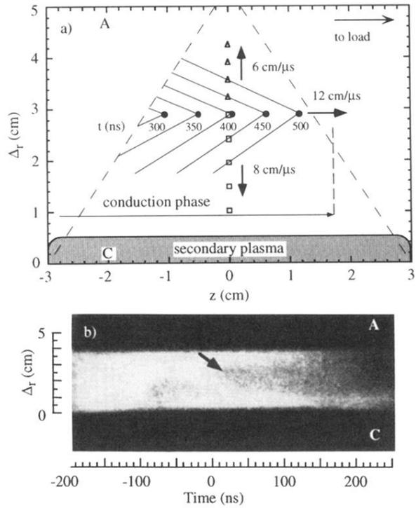
FIG. 4. (a) Reconstruction of the density maximum propagation through the plasma. Dashed lines indicate the initial plasma boundary. Moments of the peak maximum arrival are referred to the start of the upstream current. (b) Visible streak picture of the plasma (gun axis). The arrow points to the wedge front. Zero time corresponds to the 10% amplitude of the load current.
