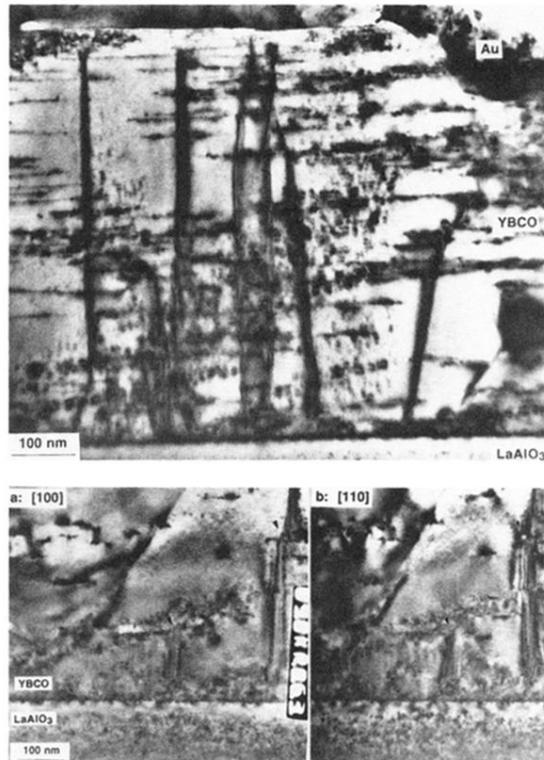
FIG. 3. (Top): Low-magnification cross-section TEM image of YBCO film grown on miscut  $\text{LaAlO}_3$ . (Bottom): Two views of the same columnar defect from orientations  $45^\circ$  apart. Gold was evaporated on the YBCO film as an electrical contact for  $J_c(H, \theta)$  measurements.
