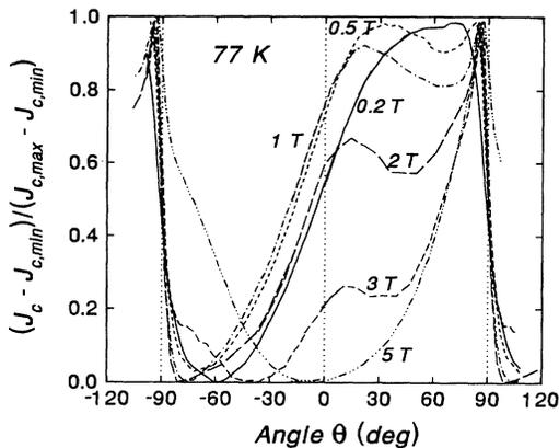
FIG. 2. Normalized  $J_c(H, \theta)$  [see Eq. (1)] for the YBCO/(1.6° miscut  $\text{LaAlO}_3$ ) specimen of Fig. 1(a), for  $H = 0.2, 0.5, 1, 2, 3,$  and  $5$  T.
