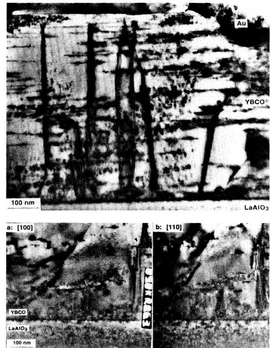
FIG. 3. (Top): Low-magnification cross-section TEM image of YBCO film grown on miscut  $\text{LaAlO}_3$ . (Bottom): Two views of the same columnar defect from orientations  $45^\circ$  apart. Gold was evaporated on the YBCO film as an electrical contact for  $J_c(H, \theta)$  measurements.
