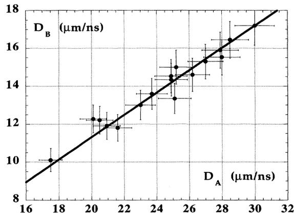
FIG. 3. Experiments with aluminum-gold targets. The shock velocity in gold,  $D_B$ , is plotted versus the shock velocity in aluminum. Error bars are 4.5% and 6% for aluminum and gold, respectively. The solid line represents the theoretical SESAME data.
