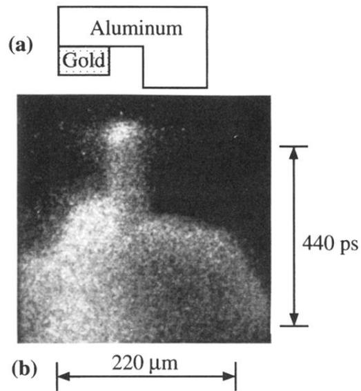
FIG. 2. Experiment on a double-step target. Optical smoothing is realized with PZP's giving a measured focal FWHM spot diameter of  $400\ \mu\text{m}$ . (a) Sketch of the target; the aluminum base thickness is  $9.5\ \mu\text{m}$ , the steps of aluminum and gold are  $4.25$  and  $1.85\ \mu\text{m}$ , respectively. (b) Streak camera record of visible light emitted by the rear side of the target.
