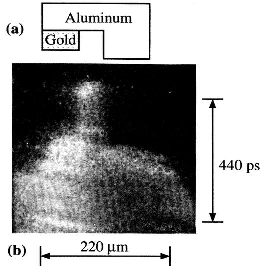
FIG. 2. Experiment on a double-step target. Optical smoothing is realized with PZP's giving a measured focal FWHM spot diameter of  $400 \mu\text{m}$ . (a) Sketch of the target; the aluminum base thickness is  $9.5 \mu\text{m}$ , the steps of aluminum and gold are 4.25 and  $1.85 \mu\text{m}$ , respectively. (b) Streak camera record of visible light emitted by the rear side of the target.
