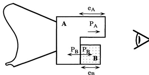
FIG. 1. Double-step targets with common base and two steps of different materials,  $A$  and  $B$ . From the shock traveling time in these steps, obtained with a visible streak camera, the shock velocities,  $D_A$  and  $D_B$ , are determined.  $P_A$  and  $P_B$  are the corresponding pressures.
