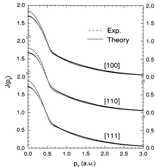
FIG. 1. Measured Compton profiles along the three principal symmetry directions are compared with the corresponding theoretical profiles broadened to reflect experimental resolution.
