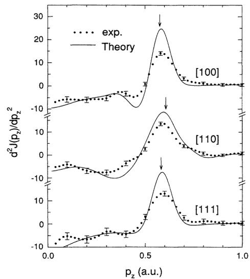
FIG. 3. Same as Fig. 1, except that this figure shows the second derivative  $d^2J/dp_z^2$ . Arrows denote the positions of the theoretical Fermi surface radii.
