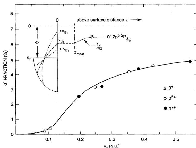
FIG. 3.  $O^-$  scattered charge fractions for  $O^{1+}$ ,  $O^{5+}$ , and  $O^{7+}$  incident ions as a function of projectile velocity under the conditions of Fig. 1—the solid line is drawn to guide the eye; inset schematically indicates  $O^-$  formation mechanism.
