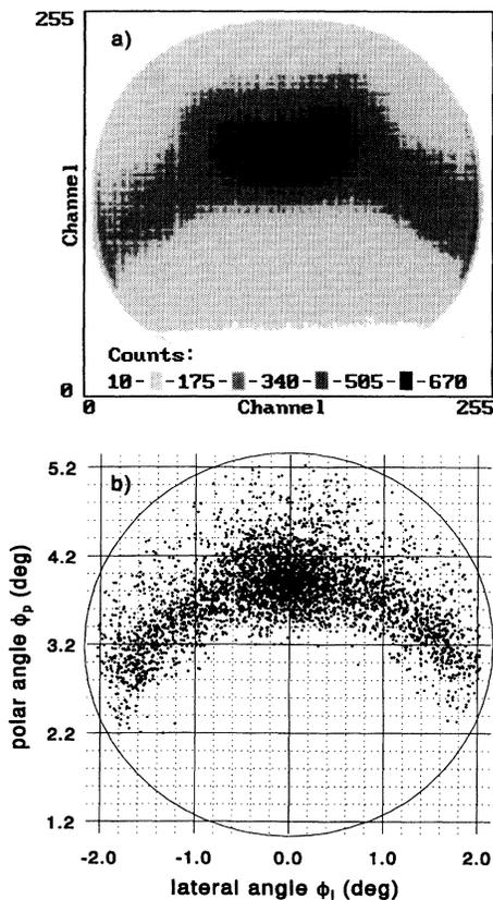
FIG. 1. Comparison of the measured (top) and simulated (bottom) scattered projectile intensity distribution on the PSD for 3.75 keV/amu  $O^{8+}$  incident on Au(110) along the  $\langle 1\bar{1}0 \rangle$  direction at  $1.8^\circ$ , showing the characteristic “banana”-shaped angular scattering distribution indicative of surface channeling.
