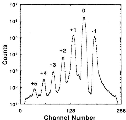
FIG. 2. Measured scattered projectile charge fractions vs initial oxygen projectile charge state for the experimental conditions of Fig. 1. Lateral scattering angle range  $-0.15^\circ$  to  $+0.15^\circ$ , polar scattering angle range  $2.0^\circ$  to  $4.5^\circ$ .
