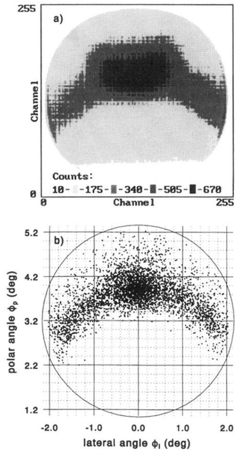
FIG. 1. Comparison of the measured (top) and simulated (bottom) scattered projectile intensity distribution on the PSD for 3.75 keV/amu  $O^{8+}$  incident on Au(110) along the  $\langle 1\bar{1}0 \rangle$  direction at  $1.8^\circ$ , showing the characteristic “banana”-shaped angular scattering distribution indicative of surface channeling.
