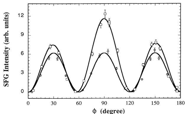
FIG. 3. Variation of SFG intensity with azimuthal angle  $\phi$  at  $2800\text{ cm}^{-1}$  in *sss* polarization for ODT/Au(111) ( $\diamond$ ) and air/Au(111) ( $\square$ ). The solid lines are the theoretical fit based on  $(1 \times 1)C_{3v}$  structure for ODT/Au(111) and  $(\sqrt{3} \times 23)$  structure for air/Au(111).
