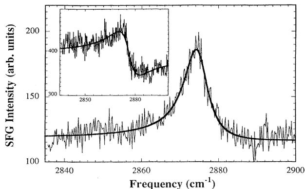
FIG. 1. SFG spectrum of ODT/Au(111) in *ppp* polarization at  $\phi = 37^\circ$ . Inset: The same spectrum at  $\phi = 7^\circ$ . The marked difference in the spectra results from the dependence of the relative phase between the nonresonant and resonance signals on the azimuthal angle  $\phi$ .
