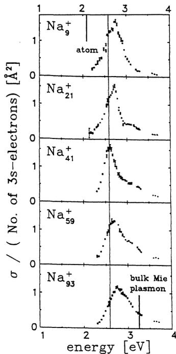
FIG. 1. Optical response of spherical sodium cluster ions. One large maximum is observed, accompanied by a shoulder on the high energy side. The vertical line gives the peak position for  $j = 41$ , indicating the blueshift for smaller and larger clusters. The positions of the atomic and the Mie resonance are also indicated.
