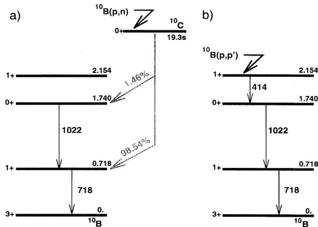
FIG. 2. (a) Decay scheme of  $^{10}\text{C}$  observed in the relative yield measurement. The ground state and 2.154 MeV levels both have negligible direct feeding in the decay [9]. (b) Main deexcitation route for the 2.154 MeV level populated in beam for the relative efficiency measurement.
