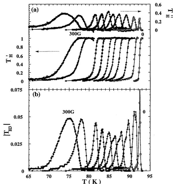
FIG. 1. The temperature dependence of the fundamental broadband transmittivity (a) and modulus of third harmonic transmittivity (b) of sample 1 ( $B_\Phi = 200$  G) in applied fields between 0 (far right) to 300 G (far left), measured using an ac field of 2.1 Oe and  $f = 7.75$  Hz.
