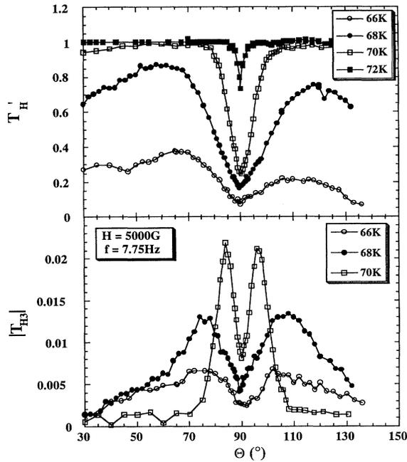
FIG. 3. Angular dependence of the fundamental (a) and third harmonic (b) transmittivity of sample 2, measured at  $f = 7.75$  Hz in a field of 5000 G. The angle  $\Theta = 0$  corresponds to the  $H \parallel ab$ ,  $\Theta = 90^\circ$  means that the field is parallel to the sample  $c$  axis and to the columnar defects.
