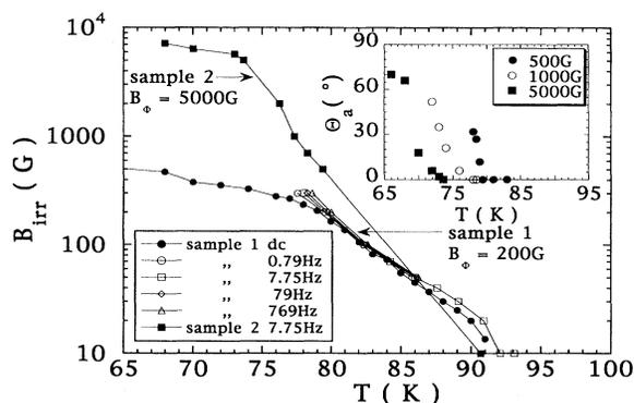
FIG. 2. The irreversibility lines  $B_{irr}$  (at several frequencies) and  $B_{dc}$  as determined by the onset of the third harmonic transmittivity and closing of the  $\Delta H_s$  loop, respectively, for both samples 1 and 2. The inset shows the accommodation angle  $\Theta_a$ , also determined by the onset of  $T_{H3}$  (sample 2,  $B_\Phi = 5$  kG).
