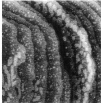
FIG. 4. 6.3 \times 6.3 \mu\text{m} area near boundary between sectors 2 and 3 of hillock in Fig. 3(a). Note the presence of islands on all terraces.
