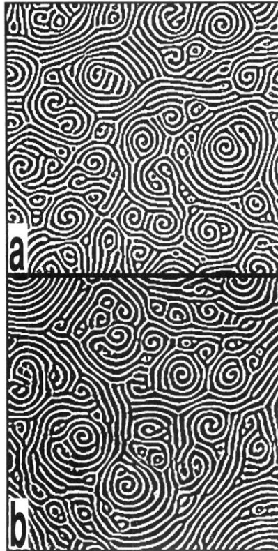
FIG. 2. Snapshots of the temperature field \theta_1 from simulations (a) at \epsilon=0.7 , Pr=1 compared with experimental results (b) ( \epsilon=0.72 , Pr=0.96 ) (with courtesy from [6]).
