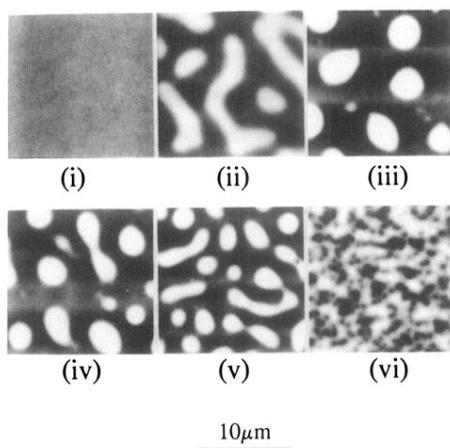
FIG. 1. AFM micrographs of homopolymer films  $\sim 100$  Å thick annealed for 24 h at 185 °C on ordered block copolymer films. (i)  $N_H = 650$ , 200–200; (ii)  $N_H = 650$ , 91–590–91; (iii)  $N_H = 2200$ , 200–200; (iv)  $N_H = 6700$ , 200–200; (v)  $N_H = 6700$ , 510–540; (vi)  $N_H = 6700$ , 800–870.
