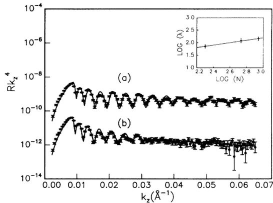
FIG. 2. Neutron reflectivity data plotted as  $\log(Rk_z^4)$  vs  $k_z$  ( $\text{\AA}^{-1}$ ) for a *dPS* ( $N_H = 5500$ ) film, 710  $\text{\AA}$  thick, on the top of a ordered 200–200 diblock copolymer film, 720  $\text{\AA}$  thick; (a) unannealed (b) after annealing for 5 h at 172  $^\circ\text{C}$ . Inset:  $\log(\lambda)$  vs  $\log(N)$  for homopolymer films of  $N_H = 5500$  and 6700, on the ordered block copolymer surfaces.
