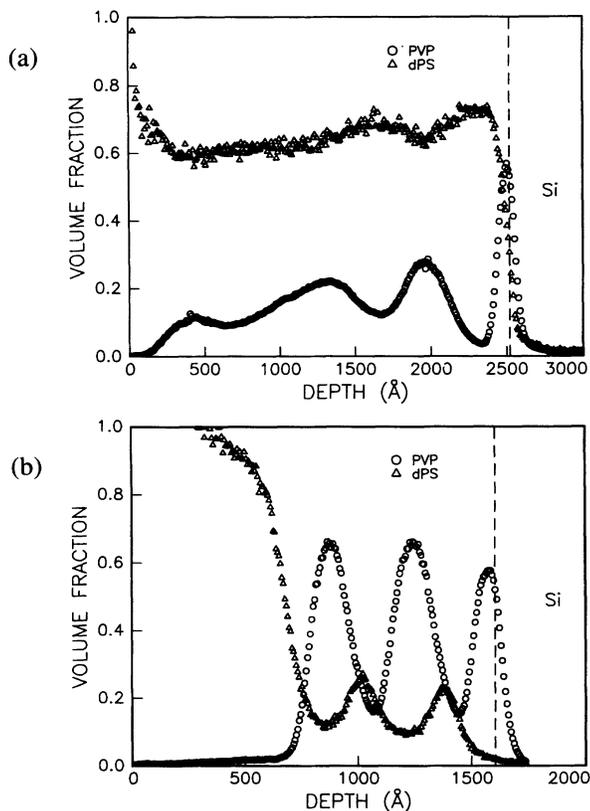
FIG. 3. The volume fraction vs depth profile as measured by SIMS of *dPS* homopolymer films ( $\Delta$ ) after annealing for 5 h at 172 °C on a previously ordered 200–200 block copolymer substrate (PVP volume fraction designated by  $(\circ)$ ); (a)  $N_H = 270$ , (b)  $N_H = 1040$ .
