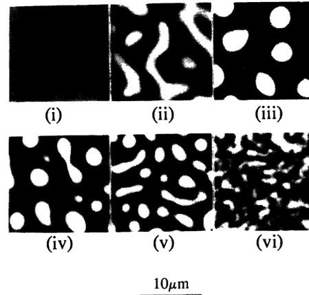
FIG. 1. AFM micrographs of homopolymer films  $\sim 100$  Å thick annealed for 24 h at 185 °C on ordered block copolymer films. (i)  $N_H = 650$ , 200–200; (ii)  $N_H = 650$ , 91–590–91; (iii)  $N_H = 2200$ , 200–200; (iv)  $N_H = 6700$ , 200–200; (v)  $N_H = 6700$ , 510–540; (vi)  $N_H = 6700$ , 800–870.
