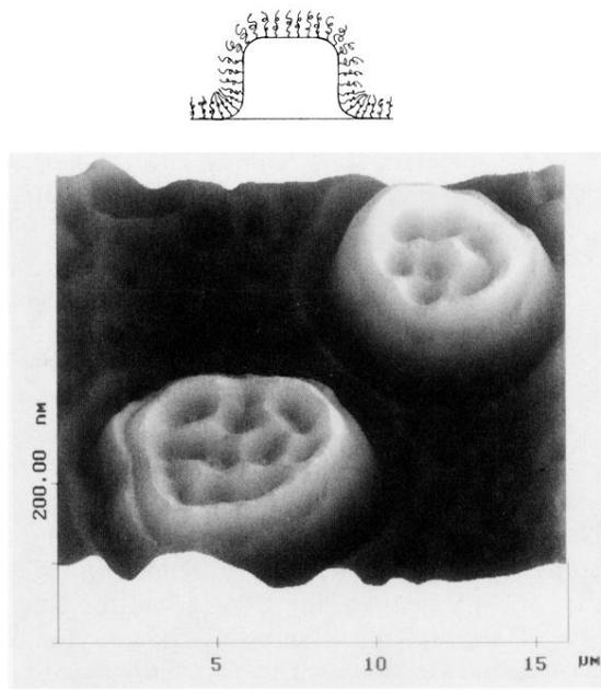
FIG. 4. AFM micrograph of the dewetting structure of a *h*PS film,  $N_H = 6700$ , around islands on the surface of a 510–540 ordered diblock copolymer layer. Inset: schematic of the brush surface around the periphery of an island.
