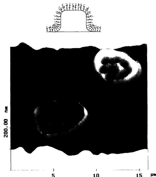
FIG. 4. AFM micrograph of the dewetting structure of a *hPS* film,  $N_H = 6700$ , around islands on the surface of a 510–540 ordered diblock copolymer layer. Inset: schematic of the brush surface around the periphery of an island.
