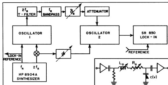
FIG. 2. A schematic of the experiment (see text). Inset: a schematic of one of the nonlinear oscillators.
