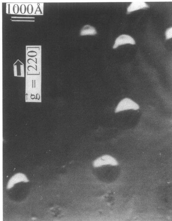
FIG. 1. Strained Ge island on Si(001). The “black-white” contrast is typical of the weak-beam dark field condition on the [220] reflection used to image the island. This microstructure was obtained after 30 min of growth.
