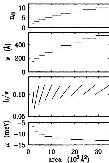
FIG. 3. Calculated island properties versus island size (cross-sectional area), from the mean-field model described in text. From top, properties are number  $n_{dl}$  of dislocations, island width  $w$ , height-to-width ratio  $h/w$ , and chemical potential  $\mu$ , where zero corresponds to a uniform strained layer. In contrast with experiment, no islanding occurs prior to the introduction of dislocations, because the model does not include elastic strain relaxation.
