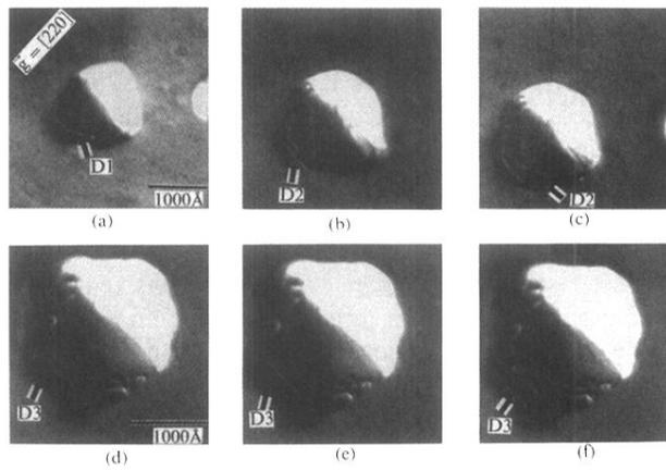
FIG. 2. Series of frames grabbed from the video recording of the growth, at the following time intervals (starting from beginning of growth). Note the change of magnification between (a)–(c) and (d)–(f). (a)  $t = 59$  min, (b)  $t = 94$  min, (c)  $t = 96$  min, and (d)–(f)  $t = 140$  min; these three pictures were taken within about 1 s of each other.
