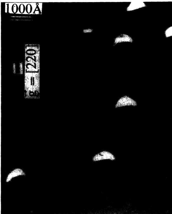
FIG. 1. Strained Ge island on Si(001). The “black-white” contrast is typical of the weak-beam dark field condition on the [220] reflection used to image the island. This microstructure was obtained after 30 min of growth.
