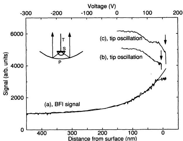
FIG. 1. Approach signals versus  $z$  piezovoltage and estimated distance from surface  $d$  for (a) BFI signal ( $\lambda = 592.187$  nm), (b), (c) tip oscillation amplitude with (c) measured 20 min after (b). All scales have the same zero. Inset: Optical schematic showing tip ( $T$ ), sample ( $S$ ) on glass hemisphere, and paraboloidal mirror ( $P$ ).
