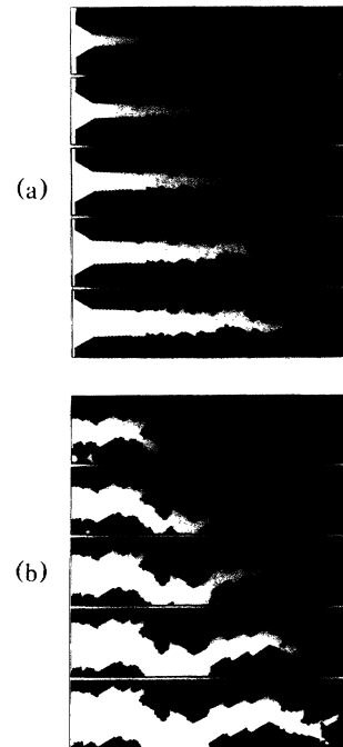
FIG. 3. (a) The onset of crack instability, in reduced time intervals of 7 and beginning at reduced time 85. (b) Late zigzag crack propagation, in reduced time intervals of 7 and beginning at reduced time 220.
