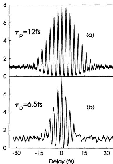
FIG. 4. Interferometric autocorrelation traces of nearly bandwidth-limited pulses (minimum-uncertainty wave packets) (a) incident on and (b) transmitted through the (HL)<sup>11</sup> sample.
