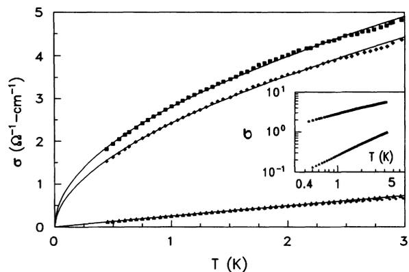
FIG. 2. Low temperature  $\sigma$  for annealed  $\text{Al}_{70.5}\text{Pd}_{21}\text{Re}_{8.5}$  samples. Lines are drawn to show power law dependence corresponding to the slope of the log-log plot for  $T < 3\text{ K}$  (inset). (■)  $\sigma \sim T^{0.55}$ , (◆)  $\sigma \sim T^{0.51}$ , for samples annealed at 940 °C for 12 h. (●) and (▲) samples with additional annealing at 600 °C for 2 h, showing  $\sigma \sim T$  (data overlap for these two samples below 2 K).
