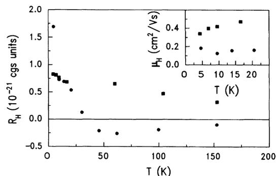
FIG. 3. Hall coefficient and Hall mobility (inset) for  $\text{Al}_{70.5}\text{Pd}_{21}\text{Re}_{8.5}$  annealed at 940 °C for 12 h (■), and annealed at 940 °C for 12 h, followed by an additional anneal at 600 °C for 2 h (●).
