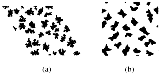
FIG. 5. Islands grown on a (a) triangular and a (b) square lattice, at identical conditions. The lattice size is 200 \times 200 in each case, and periodic boundary conditions have been imposed.
