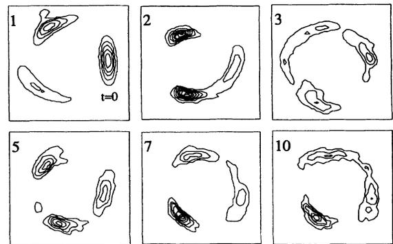
FIG. 3. Time evolution of the wave packet in the laboratory frame. Snapshots of the contour lines of the probability distribution are taken 3 times per cycle for the cycles 1, 2, 3, 5, 7, and 10. The packet starts with the smooth Gaussian shape shown in cycle 1 and moves counterclockwise.
