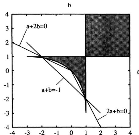
FIG. 1. The islands of stability (shaded areas) in the plane of parameters  $a$  and  $b$ . In the parabolic triangle the potential has a saddle point but the motion is stable due to an interplay of potential forces and the Coriolis force. Points lying on the three lines intersecting the triangular stability regions correspond to the gravitational three-body problem and to an atom in a circularly polarized wave.
