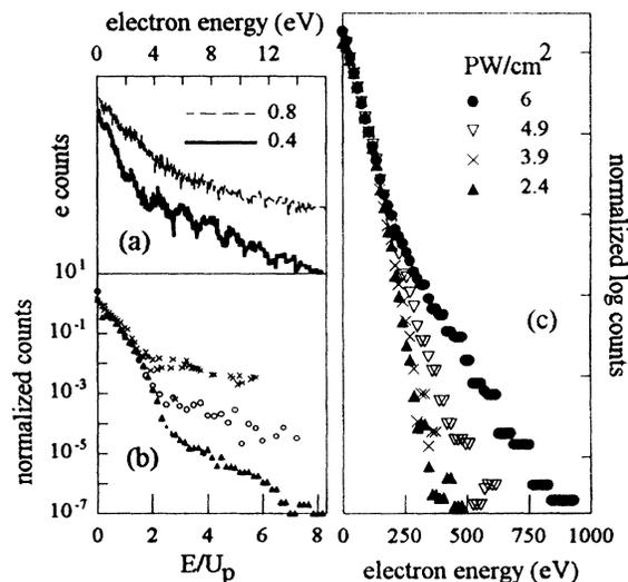
FIG. 2. Helium photoelectron spectra for 780 nm excitation. Low energy electrons plotted in (a) for 0.4 and 0.8 PW/cm $^2$ . Scaled energy,  $E/U_p$ , plot at (b) 0.2 (crosses), 0.4 (circles), and 1.0 (triangles) PW/cm $^2$ . The value of  $U_p$  is defined by the laser's peak intensity. Plot (c) shows the high energy electron tail (solid circles) resulting from the sequential formation of  $He^{2+}$ .
