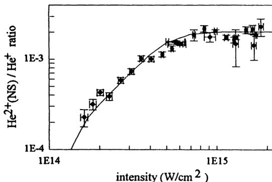
FIG. 3. Intensity dependence of  $\text{He}^{2+}(\text{NS})/\text{He}^+$  ratio. Error bars indicate 1 standard deviation. Solid line is calculated; see text for details. The measured intensities are multiplied by 1.15.
