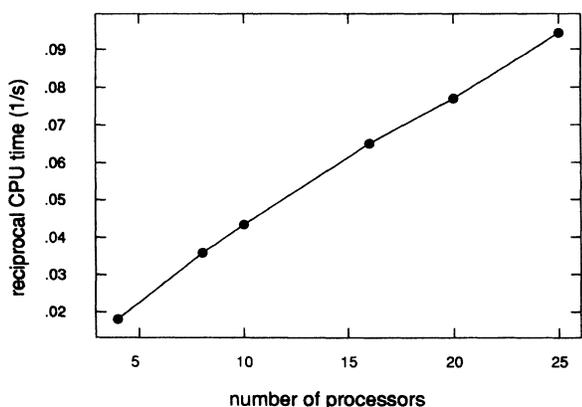
FIG. 3. Execution speed as a function of the number of processors on an IBM SP1. The system considered is a 1000-carbon atom cell.
