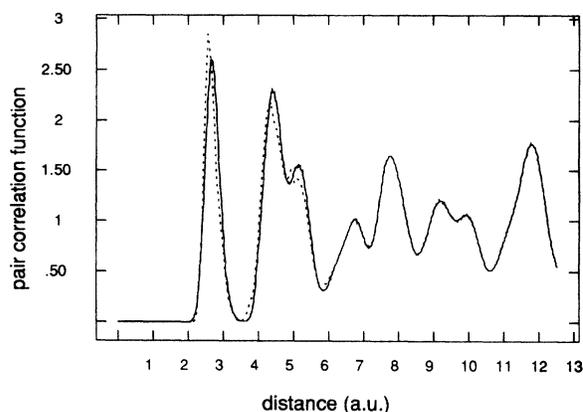
FIG. 4. Particle-particle correlation function  $g(r)$  for solid high-density carbon at 6500 K. The dashed lines represent the CPMD results of Ref. [7].
