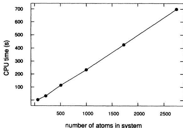
FIG. 2. CPU time on an IBM RS6000/550 workstation to calculate  $E_{bs}$  and HF forces with the present method for cells containing carbon atoms.
